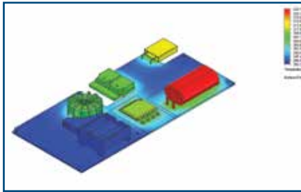
Temperature distribution from a CFD analysis in SOLIDWORKS Flow Simulation
